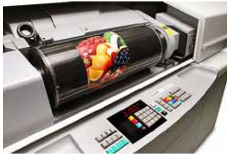
DRUM SCANNERS wrap the image on a drum, regardless of its size.
