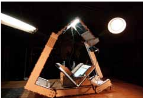
DIY BOOK SCANNER. Graduate student Daniel Reetz made this book scanner in 3 days, for about $300. He lashed together two lights, two Canon Powershot A590 cameras, a few pieces of acrylic and some wood. It's fast enough to scan a 400-page book in about 20 minutes. To use it, he simply loads in a book and presses a button, then turns the page and presses the button again. Each press of the button captures two pages, and when he's done, software on Reetz's computer converts the book into a PDF file. The Reetz DIY book scanner isn't automated—you still need to stand by it to turn the pages. But it's fast and inexpensive. His how-to guide is available online.
